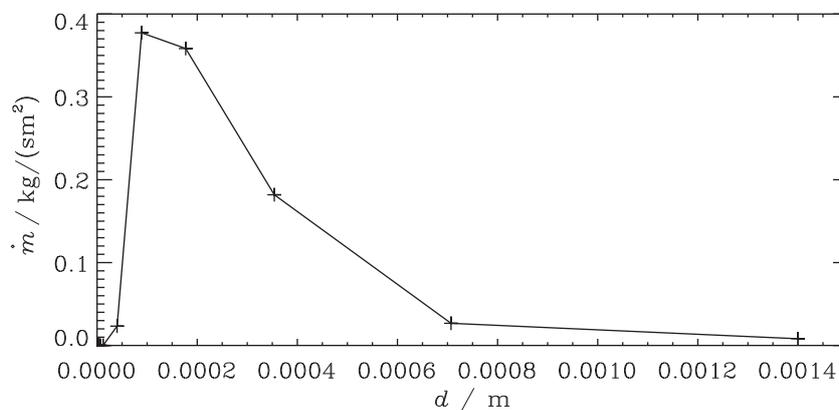
**Fig. 6.** The total specific rate of mass impactation on the front side of all the tubes in a tube row, per tube length.
