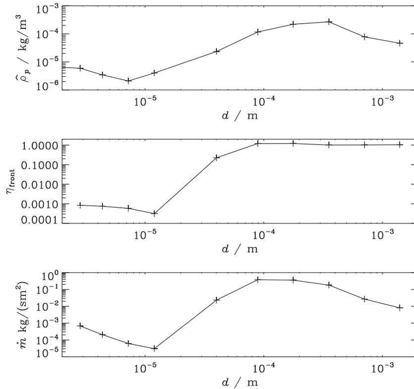
**Fig. 5.** The upper plot shows the mass density for different particle sizes, while the middle plot shows the total impact efficiency. Finally the lower plot shows the specific rate of mass impactation on the front side of the tubes, per tube length, summed over all tubes in a tube row. The values result from a combination of simulation data and measurements from the MSWI in Schweinfurt, Germany.
