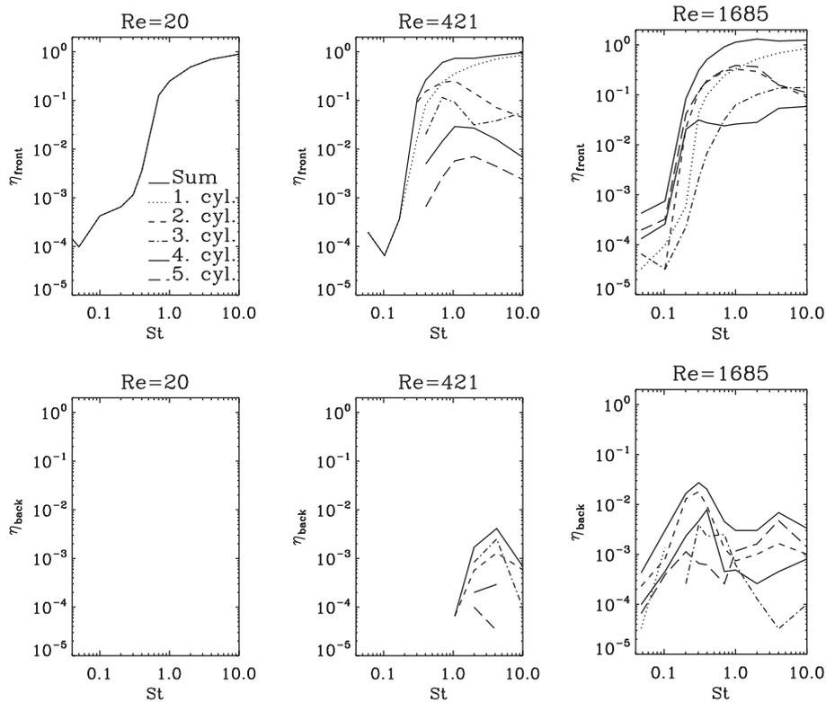
**Fig. 2.** Front side (upper plots) and back side (lower plots) impact efficiency as a function of Stokes number for different Reynolds numbers. Here both the impact efficiencies for the sum of all the five tubes (solid line) and for each individual tube are shown.
