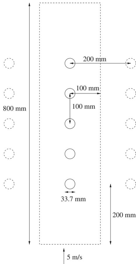
**Fig. 1.** Here the geometry of the first five tubes of the GKS plant is shown. The dashed rectangle corresponds to the domain of the simulations, where the lower boundary is the inlet and the upper boundary is the outlet. The side boundaries are periodic, mimicking an infinite number of tube rows on each side of the domain as illustrated by the two dashed tube rows on each side of the rectangle.
