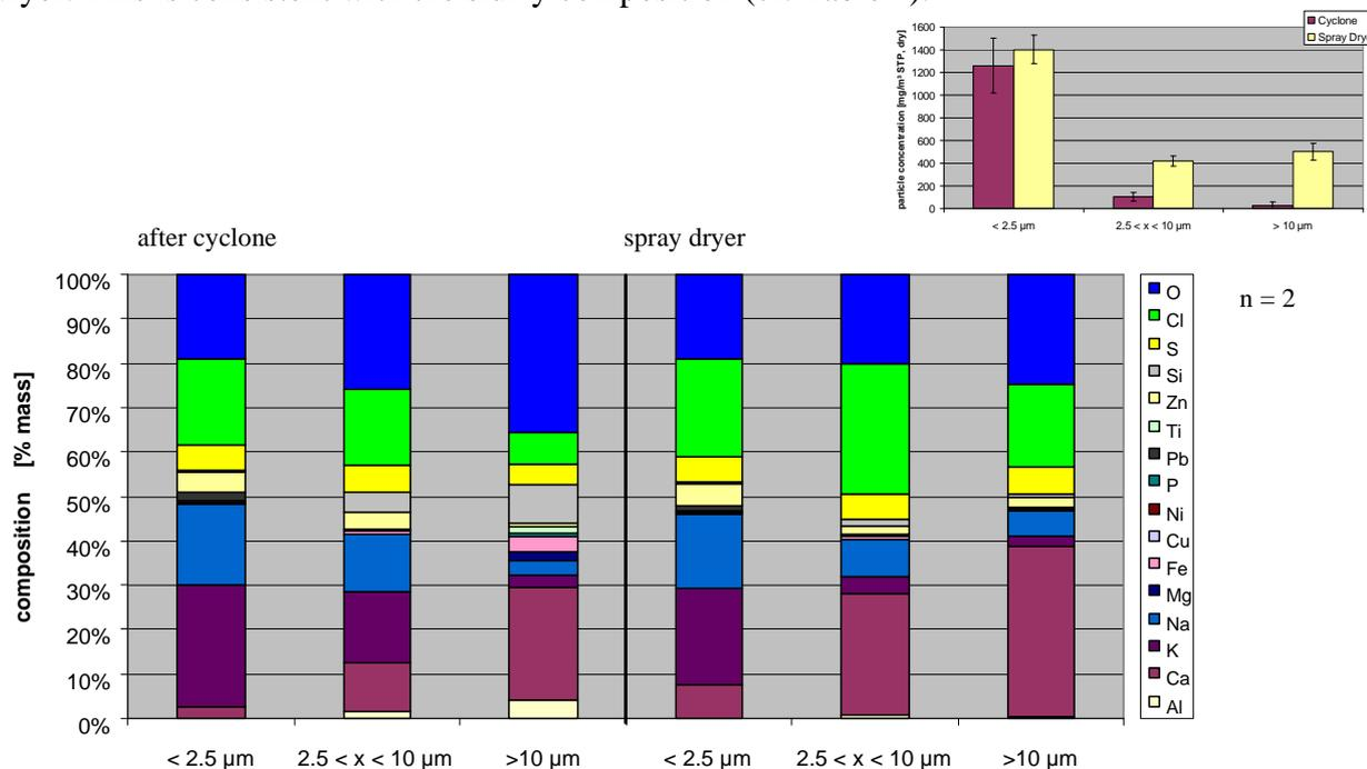
Figure 14: Change in particle composition in the spray dryer
