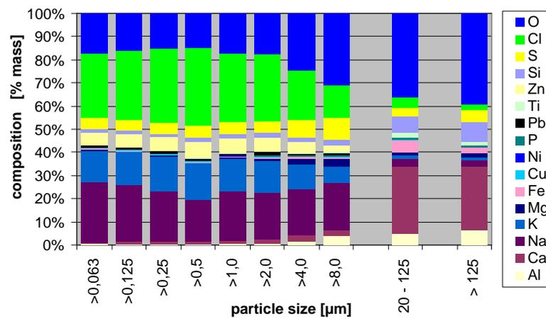
**Figure 13: Typical composition of particles in the 4<sup>th</sup> pass and at the boiler exit [Warnecke and Nordsieck, 2008, adapted]**
