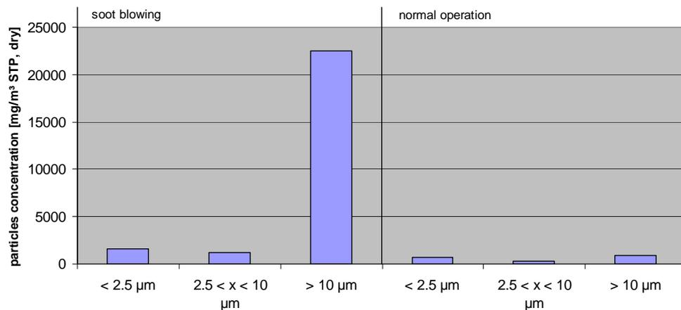
**Figure 17: Effect of soot blowing on dust particle concentration and size distribution**
