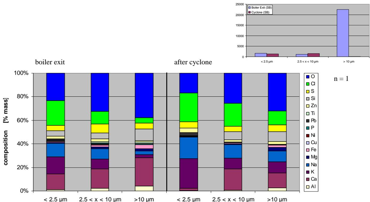
**Figure 18: particle composition before and after the multiclone during soot blowing**
