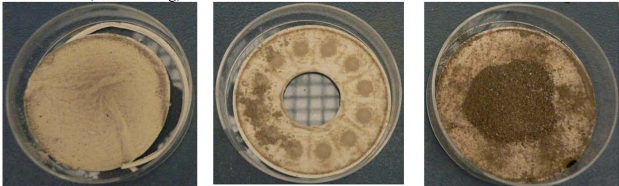
b: boiler exit (normal operation, low impactor load)
