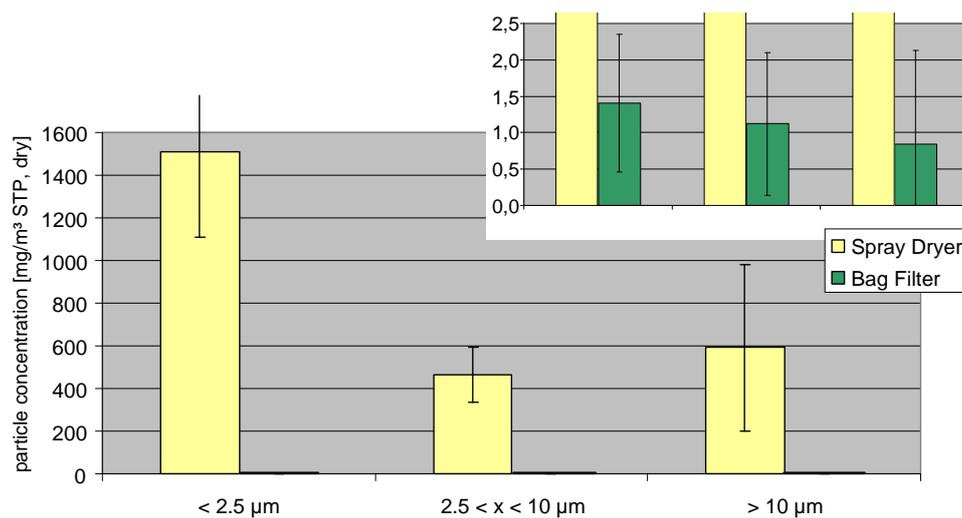
**Figure 10:** Particle size distribution before and after the bag filter (“spray dryer” and “bag filter”, respectively), the ordinate in the small figure is adapted to show the amount of particles behind the filter.
