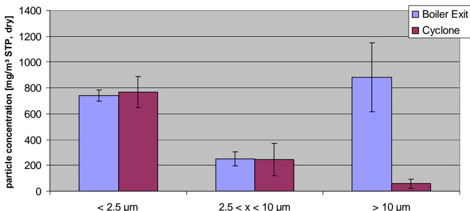
**Figure 8:** Particle size distribution before (boiler exit, n=2) and after the multicyclone (cyclone, n=2)
