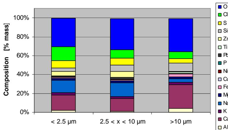
**Figure 3: Mean dust composition at the boiler exit (without soot blowing, n=2)**
