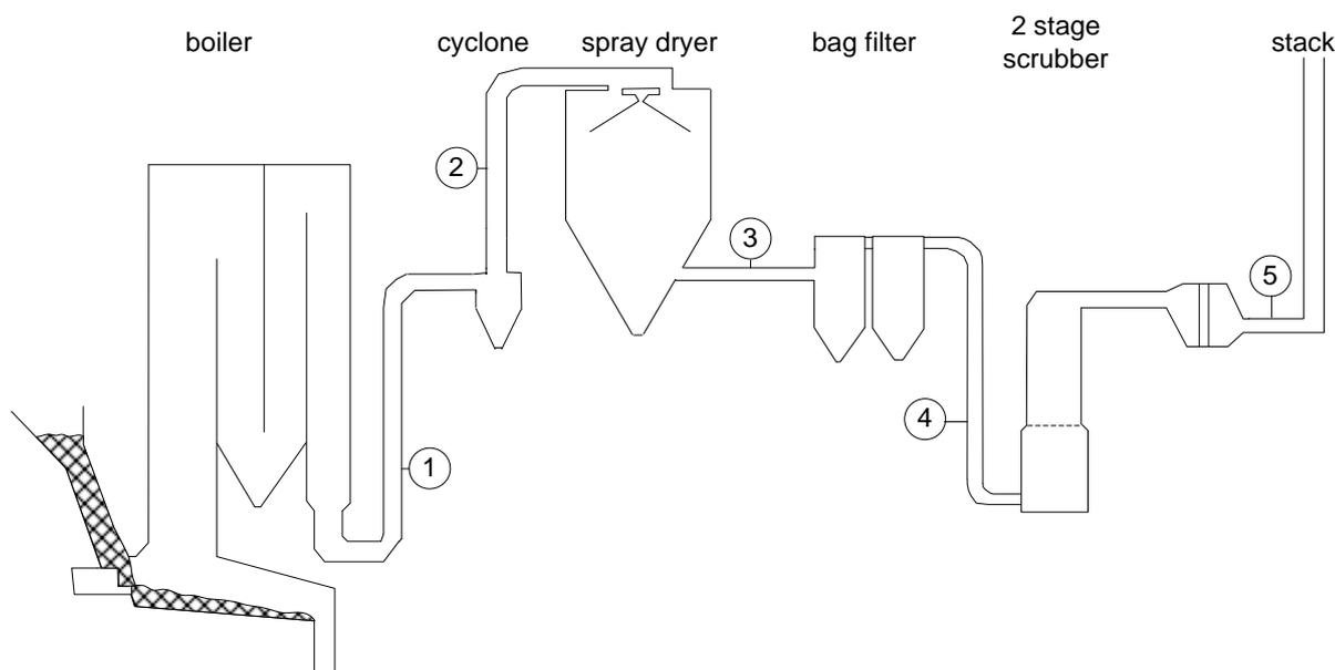
**Figure 1: Sampling positions on the flue gas treatment system**
