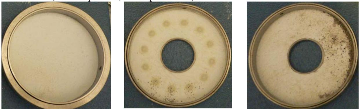
**Figure 2: Examples of impactor stages after sampling**
