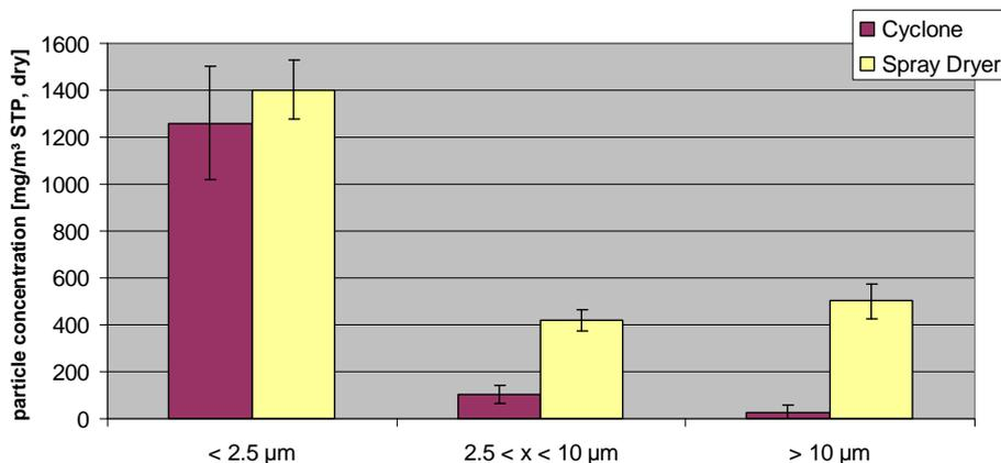
**Figure 9:** Particle size distribution before and after the spray dryer (“cyclone” and “spray dryer”, respectively)
