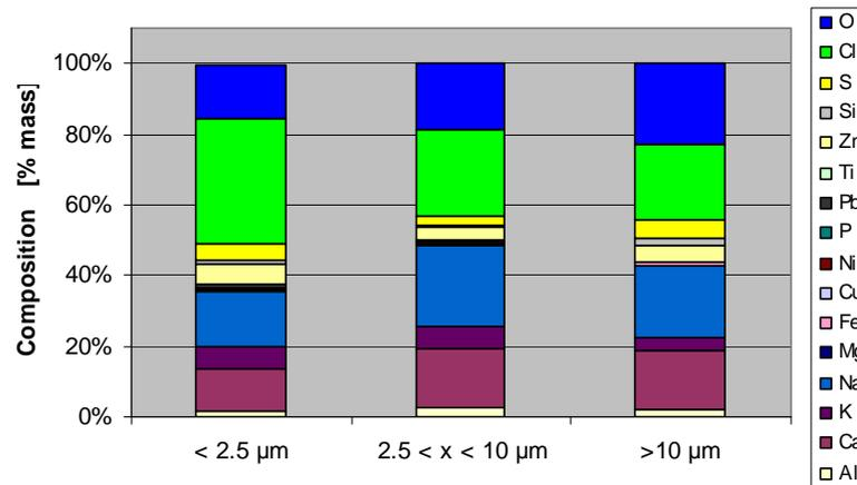
**Figure 6: Mean dust composition after the bag filter (without soot blowing, n=6)**
