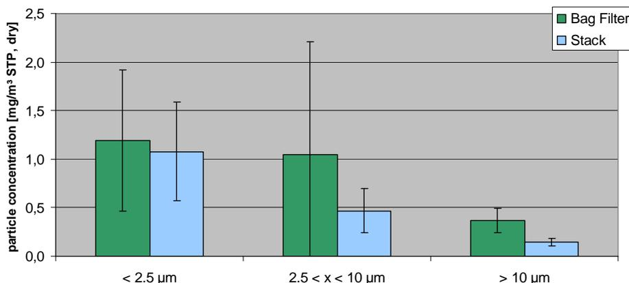
**Figure 11: Impact of the 2 stage scrubber unit on the dust particle size distribution**
