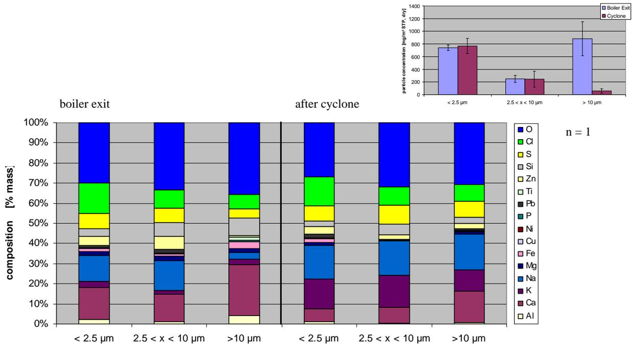
**Figure 12: Change in particle composition in the multiclone**
