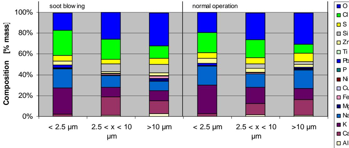
**Figure 19: Particle composition after the multicyclone during soot blowing compared to the composition at normal operation**
