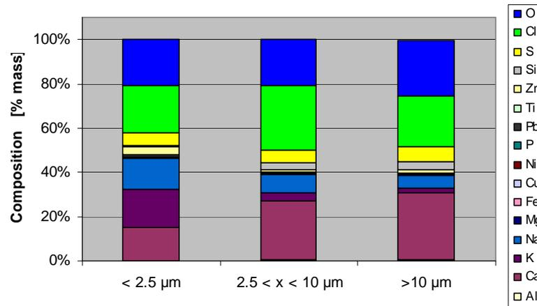
**Figure 5: Mean dust composition after the spray dryer (without soot blowing, n=6)**
