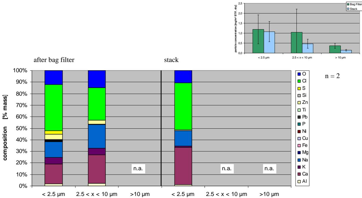
Figure 16: Composition of dust particles before and after the 2 stage scrubber (n.a. = to small sample to analyse)
