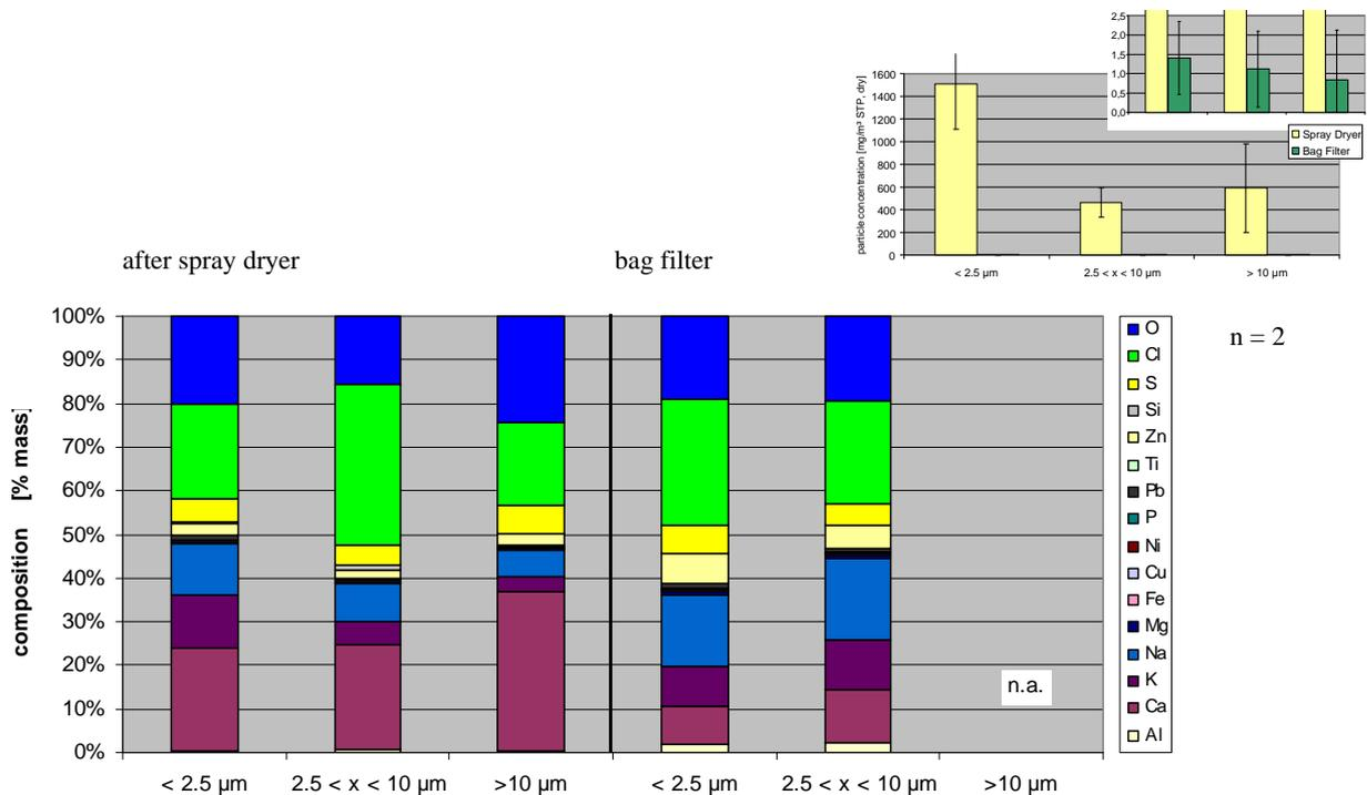
Figure 15: Change in particle composition in the bag filter (n.a. = to small sample to analyse)
