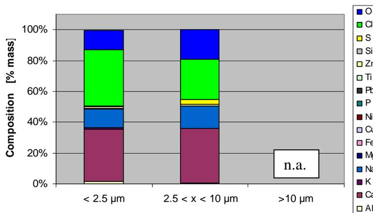
**Figure 7: Mean dust composition at the stack, i.e. after scrubber, demister and reheater (without soot blowing, n=3) (sample of particles > 10 µm to small to analyse)**
