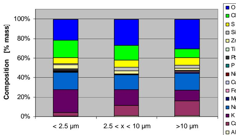
**Figure 4: Mean dust composition after the multiclone (without soot blowing, n=6)**
